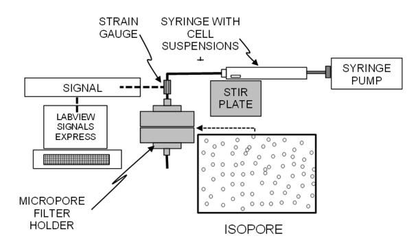
Figure 1 - Representative image of the micropore filtration setup
